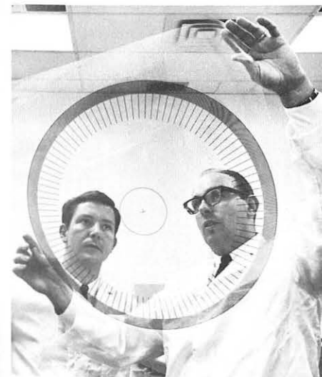
Artwork produced by a high-precision plotter driven automatically by computer commands is examined by draftsmen. The mask—used to make miniaturized encoder discs for circuit clocking—is one of many diverse applications of the experimental program.
